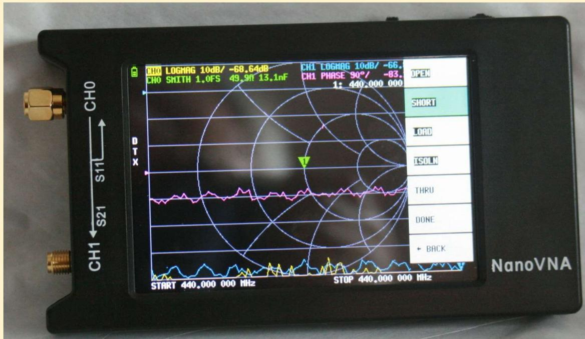
Calibration must be redone if the cable extensions or the feed through are used. The reason is that these change the timing delays by a few pico seconds which affect the testing results.
