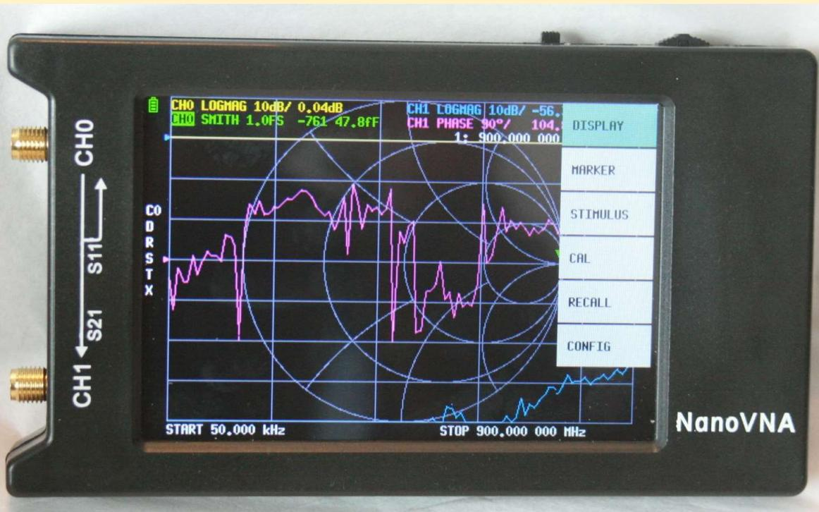
The screen displays the traces that are available for circuit analyzation. The most recognizable is the Smith Chart. The other traces represent various programmable inputs from the two ports.
