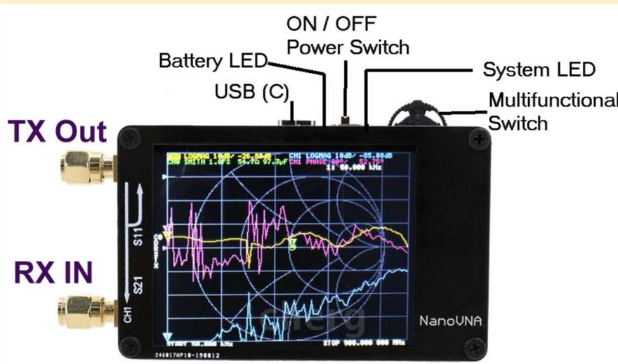
The upper socket is the transmit port (CH0) and is also the channel for S11 measurements (reflection).
