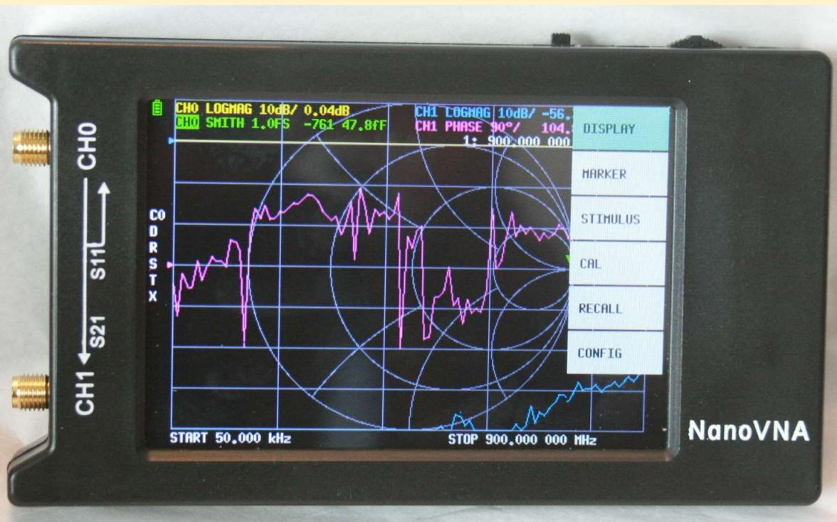
The unit contains a low level transmitter with a frequency range of 50 KHz to 300 MHz. Output is on CH0. Output frequency range is programmable and displayed at the bottom of the screen.
